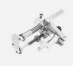
For the reliable removal of the oxide layer on spigot fittings. Additionally it is also possible to scrape HDPE and PE-Xa-pipes (maximum along half length of couplers d 710). Scraper blade made of carbide for a long life. Even swarf removal thanks to a spring-loaded scraper blade and automatic feed. Includes a replacement blade. The tool is delivered in a transport box.
