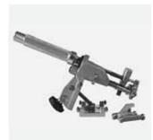
For the reliable removal of the oxide layer of HDPE and PE-Xa pipes. Scraper blade made of carbide with 2 edges (twice the service life). Consistent swarf removal due to spring mounted scraper blade and automatic feed. With quick adjustment of the scraping length and exchangeable clamping slide for the dimensions d 75 - d 225 and d 250 - d 400. The tool is delivered in a transport box.
