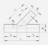
HD-PE long spigot fitting for installation with FRIAFIT electrofusion coupler. Pipe colour black with bright inner surface (according to availability)
