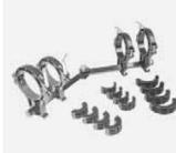
Alignment clamp with angle adjustment (45°/90°) and two clamping elements for heating coil fusion couplers, reducers, and 45° and 90° elbows d 63, d 90, d 125, and d 180. Reduction shells can be inserted for various sizes. Delivered in a practical carrier bag.
