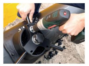
Fig 3a - Tapping with the FWFIT
