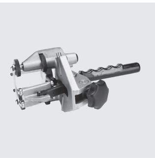
For the reliable removal of the oxide layer of HD-PE and PE-Xa pipes. Scraper blade made of carbide for a long life. Even swarf removal thanks to a spring-loaded scraper blade and automatic feed. Inclusive of a replacement scraper blade and FRIATEC maintenance spray.
