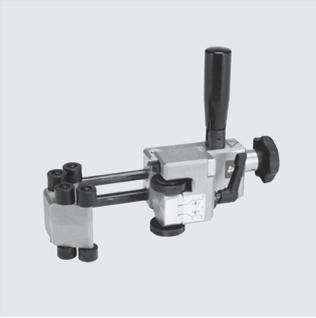
For the reliable removal of the oxide layer of HD-PE and PE-Xa pipes. Scraper blade made of carbide for a long life. Even swarf removal thanks to a spring-loaded scraper blade and automatic feed. Inclusive of a replacement scraper blade.
