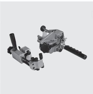
For the reliable removal of the oxide layer of HD-PE and PE-Xa pipes. Scraper blade made of carbide for a long life. Even swarf removal thanks to a spring-loaded scraper blade and automatic feed. Inclusive of a replacement scraper blade for each tool and FRIATEC maintenance spray.
