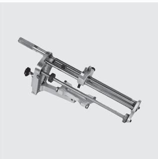
For the reliable removal of the oxide layer of HD-PE and PE-Xa pipes for half or entire coupler length. Scraper blade made of carbide for a long life. Even swarf removal thanks to a spring-loaded scraper blade and automatic feed. Inclusive of a replacement scraper blade and FRIATEC maintenance spray.
