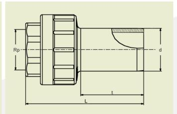
PE 100 SDR 11 Maximum working pressure 16 bar (water)/5 bar (gas)
