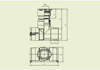
PE 100 SDR 11 Maximum working pressure 16 bar (water)
