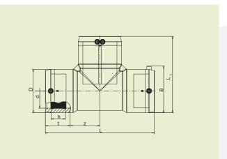
PE 100 SDR 11 Maximum working pressure 16 bar (water)/10 bar (gas)
