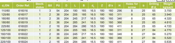
FRIALEN-Safety Fittings can be fused to pipes of SDR stages 11 to 17.6. Other SDR-stages on request. Please observe the marking directly at the product, which is mandatory. DVGW-Registration No.: DV-8606AU2249
