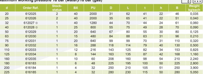
FRIALEN safety fittings can be fused to pipes SDR11 - SDR 17.6. Minimum wall thickness s min  $\geq$  3 mm. Other SDR-stages on request. Please observe the marking directly at the product, which is mandatory. DVGW-Registration Nos. DV-8601AU2248 and DV-8606AU2249
