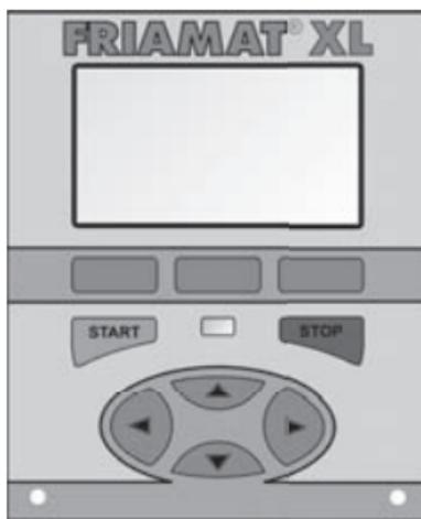
**Guide buttons:** Guide buttons are blue, are situated at the very top of the unit (directly below the graphical display) and have a grey background. The guide buttons are not labelled as their functions vary according to input and are displayed in the bottom line of the graphical display (see section 4.2 and 4.3).
