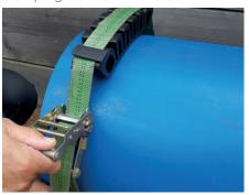
Assembly with tensioning belt.
