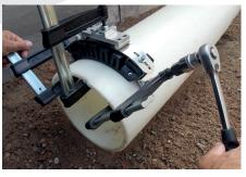
Assembly with the FRIATOOLS clamping device FIXBLOC FWFB.
