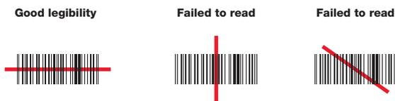
Badly printed or slightly damaged barcodes can be read in when the scanner is placed directly on the barcode and then, with the read button pressed, moved away. When the barcode is read in successfully, the device emits an acoustic signal, and a green indicator lamp lights up in the middle of the read barcode.
