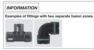
For a bifilar fitting with two separate fusion zones (two fusion barcodes), fusion of the first zone must be started via the Dashboard and at the "Fusion" button (see 5.1). This generates a new fitting ID. At the end of the process, the button "Finish fusion" opens the detail view displaying all the data relevant to the fitting.
