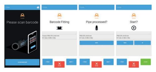
The Fusion process must be started at the FRIAMAT fusion unit or via the "Start" button in the FRIAMAT App.
